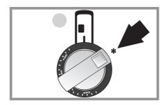
5 \* The fan only setting. The fan circulates air inside the oven but the heating element is not turned on. This setting is useful for defrosting frozen foods.
